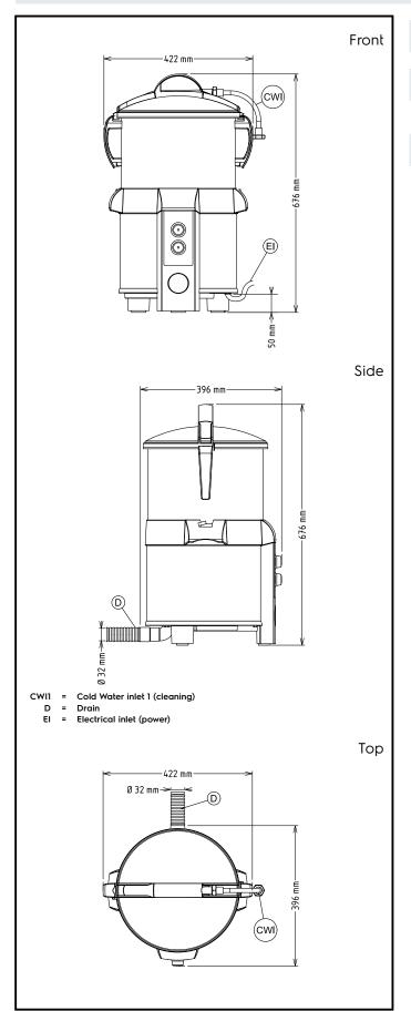
**Electric** Supply voltage: 220-240 V/1N ph/50/60 Hz Capacity: Performance (up to): 130 kg/hour Capacity: 8 litres **Key Information:** External dimensions, Width: 422 mm 396 mm External dimensions, Depth: External dimensions, Height: 676 mm Shipping weight: 25 kg
